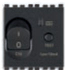
19411.16 C 16, I_{\Delta n} 10 mA, prekidna moć 3000 A - 2 modula. Dubina: 39 mm
