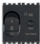
19411.06 C 6, I_{\Delta n} 10 mA, prekidna moć 1500 A - 2 modula. Dubina: 39 mm
